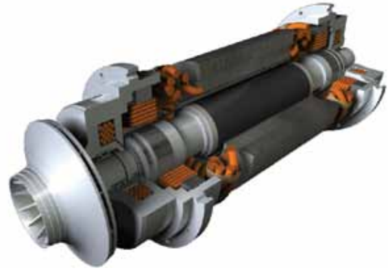
The proven permanent-magnet motor and active magnetic-bearing technology used in the YORK Navy Systems magnetic centrifugal chiller is also featured in the YMC 2 chiller.
