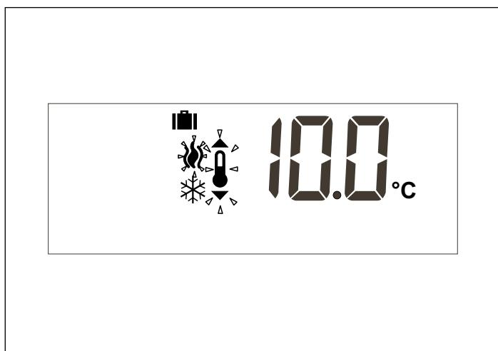
If when moving one of the set points we come to less than one degree from the following set points it will be “dragged” so as to avoid the unsuitability of the set points. When this happens, the thermostat will flash the icon of the occupation mode of this set point being dragged.
