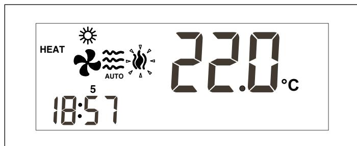
A demand is generated when the room temperature is below the programmed set point. Set point is understood as the temperature we want in the room.
