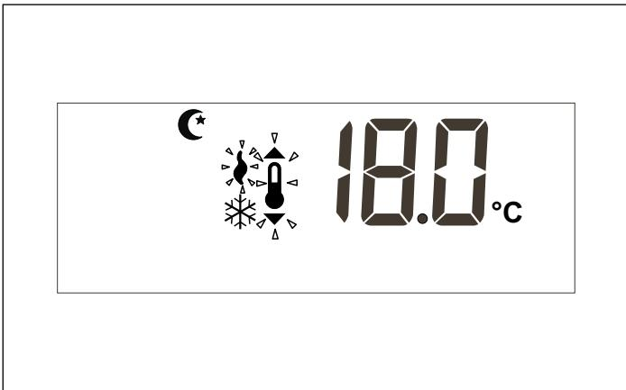
If when moving one of the set points we come to less than one degree from the following set point, it will be “dragged” so as to avoid the unsuitability of the set points. When this happens, the thermostat will flash the icon of the occupation mode of this set point being dragged.
