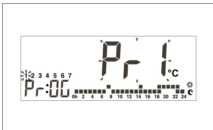
If the communication profiles are not empty, which means they are not on 24-hour stand-by, or a profile above the first six (three predefined and three user-programmable) has been selected by means of communication with the PC, profiles P7 to P12 can be selected. Should this not be the case, these profiles can neither be selected nor are displayed on screen.
