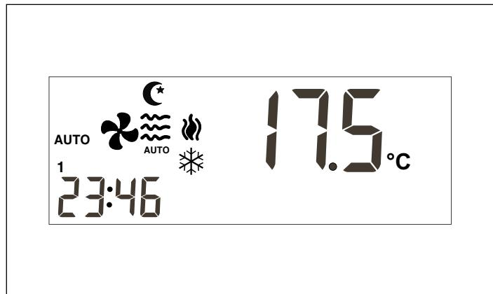
A demand is generated when the room temperature is above the cooling set point or below the heating set point. In automatic mode, room temperature is kept at a value between these two programmed set points.
